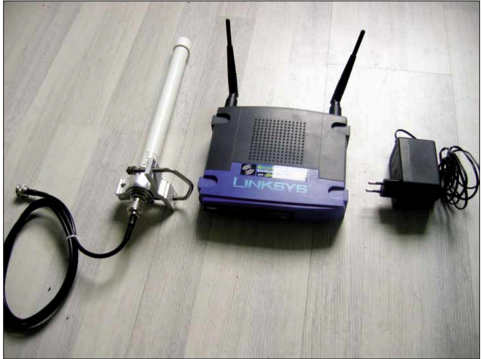
Figure 2. Components needed to install WiFi at petrol stations – a certified router (in this illustration it is a Linksys WRT 54G), an AC adapter (to the right), and a 6 dB weatherproof omni antenna with a universal attachment and an antenna cable with weatherproof connectors.
